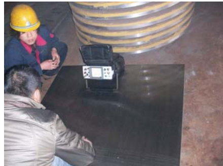
Scanning in transverse direction
